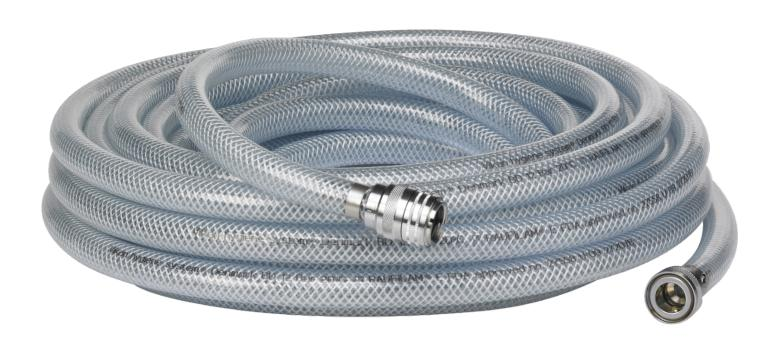
This hose is ideal for cleaning with water up to  $40^{\circ}$  C. It is equipped with a 1/2" Q-coupling in both hose ends. Water tap nipple, 0700 provided for 1/2", 3/4" and M22x1 screw thread types. Can be used with the following Vikan Q-couplings 0700, 0705 and 0712 as well as other Vikan products equipped with a 1/2" Q-nipple.
