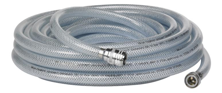
This hose is ideal for cleaning with water up to 40° C. It is equipped with a 1/2" Q-coupling in both hose ends. Water tap nipple, 0700 provided for 1/2", 3/4" and M22x1 screw thread types. Can be used with the following Vikan Q-couplings 0700, 0705 and 0712 as well as other Vikan products equipped with a 1/2" Q-nipple.
