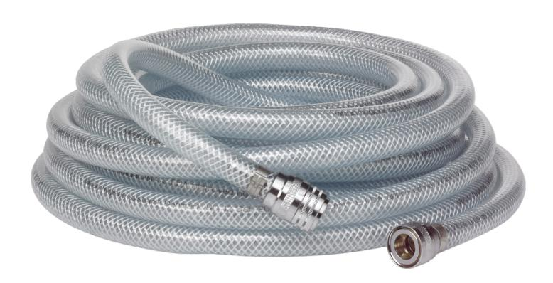
This hose is ideal for cleaning with water up to  $40^{\circ}$  C. It is equipped with a 1/2" Q-coupling in both hose ends. Water tap nipple, 0700 provided for 1/2", 3/4" and M22x1 screw thread types. Can be used with the following Vikan Q-couplings 0700, 0705 and 0712 as well as other Vikan products equipped with a 1/2" Q-nipple.
