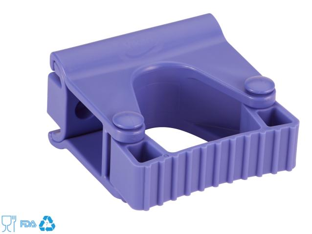
The Grip band module is designed for hanging cleaning tools without a hanging hole. Slide the Grip band module onto the supplied double-base/spacer from the left or right side. The Grip module can hold products with a diameter of 28-33 mm. The Grip band module is easy to disassemble for cleaning or replacement.
