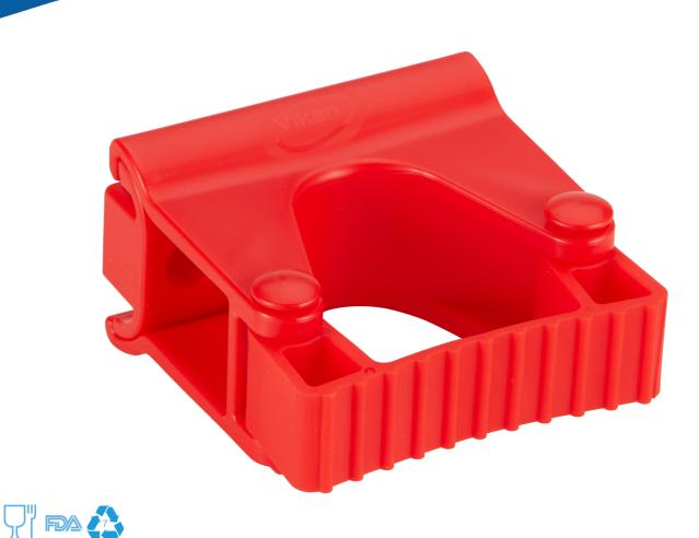
The Grip band module is designed for hanging cleaning tools without a hanging hole. Slide the Grip band module onto the supplied double-base/spacer from the left or right side. The Grip module can hold products with a diameter of 28-33 mm. The Grip band module is easy to disassemble for cleaning or replacement.
